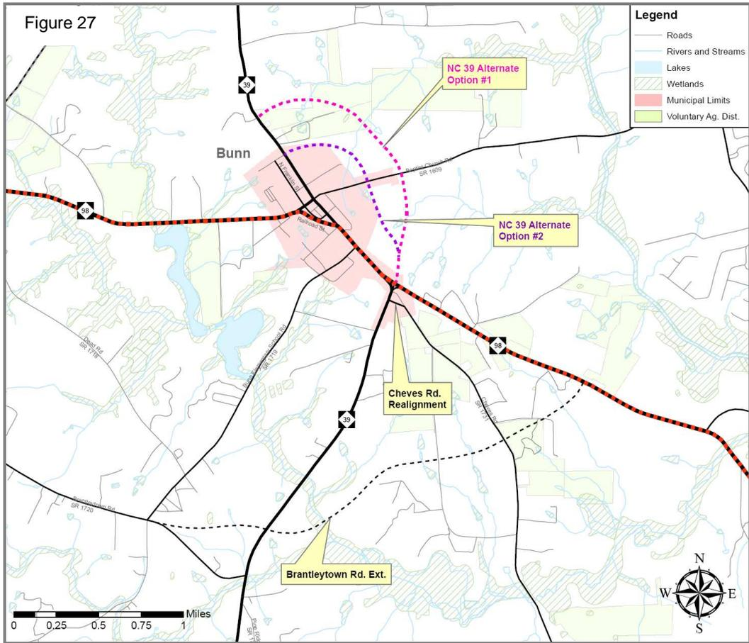
4. NC 39 Alternate #1: Constructing a new location facility east of Bunn, shown in Figure 27, outside the eastern town limits, except where it ties into NC 39/98 on the southern end, would alleviate a considerable amount of traffic in downtown Bunn.
